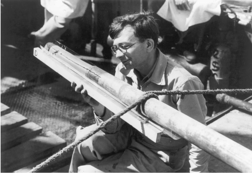
Ron Mason with piston core sample of sediments from the sea floor, on the Spencer F. Baird , 1954. (Photograph courtesy of the Scripps Institution of Oceanography, used by permission of the University of California.)
