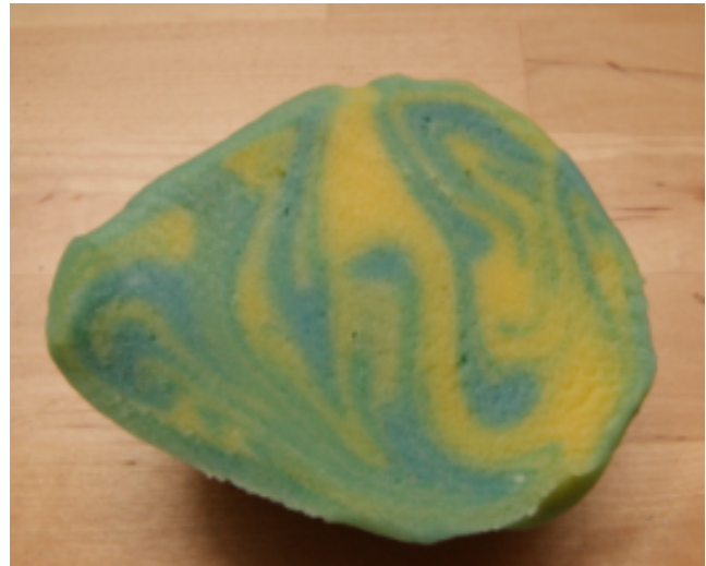
Figure 1. Example section through the dough. The yellow and blue areas have been stirred. The greener areas have been mixed.
