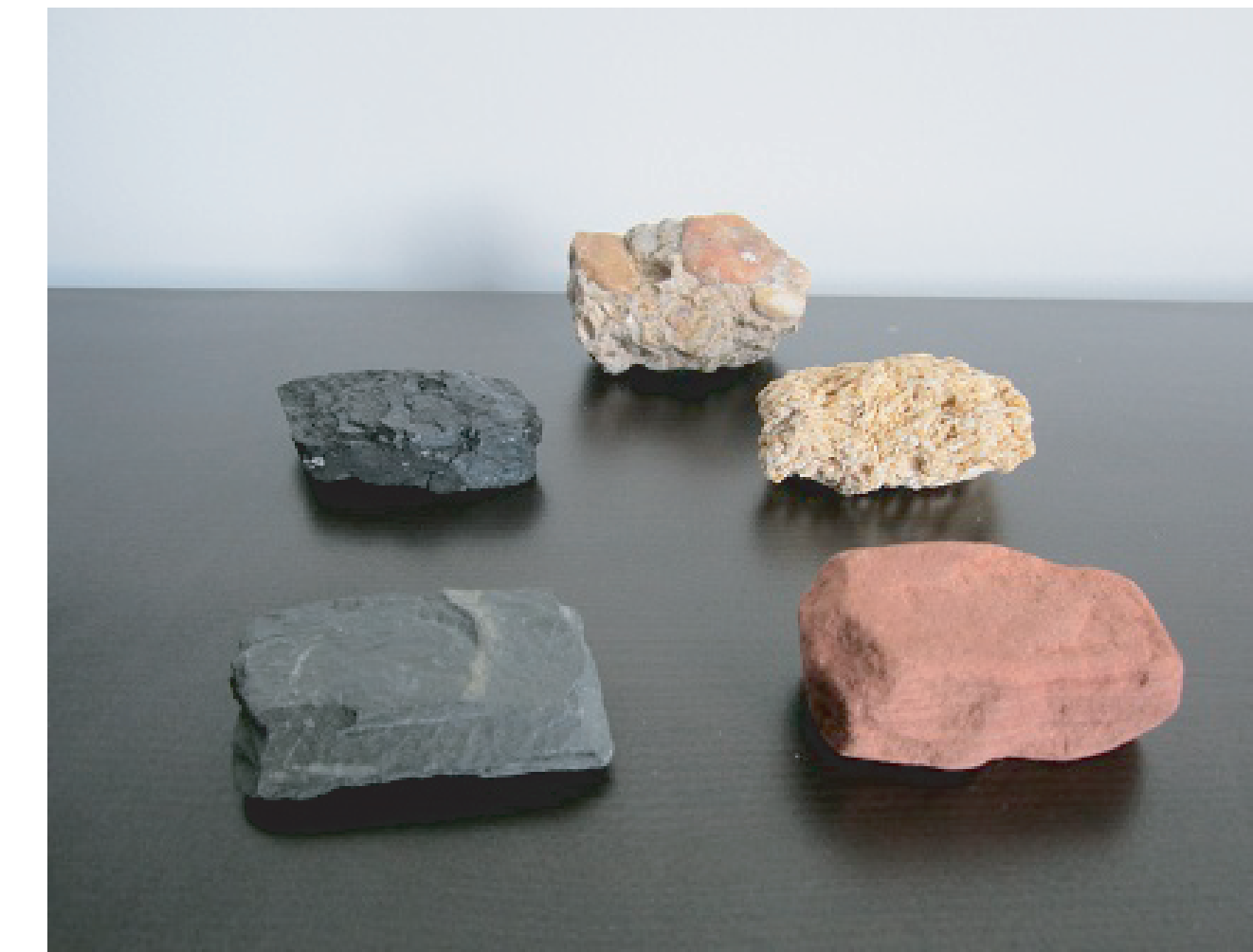
Figure 3. Photograph of select sedimentary rocks (clockwise from top: conglomerate, coquina, sandstone, shale, coal).
