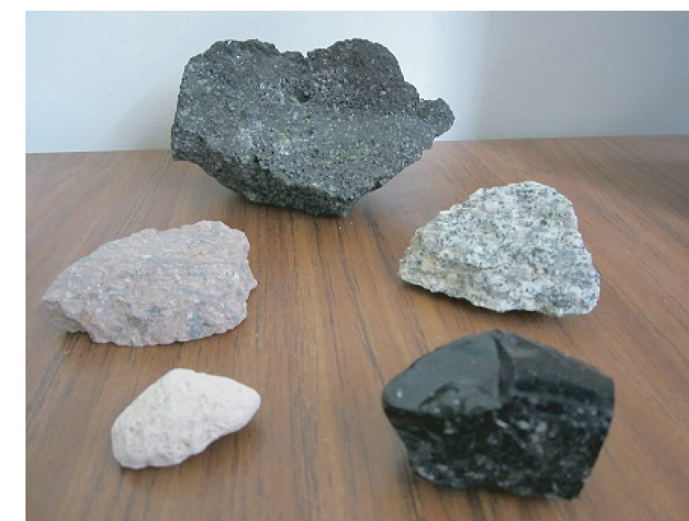
Figure 2. Photograph of a select group of igneous rock samples (clockwise from top: basalt, granite, obsidian, pumice, rhyolite)
